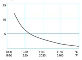
\* Holding time = time at austenitizing temperature after the tool is fully heated through.
