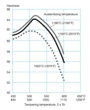
The tempering curves are obtained after heat treatment of samples with a size of  $15 \times 15 \times 40$  mm, cooling in forced air. Lower hardness can be expected after heat treatment of tools and dies due to factors like actual tool size and heat treatment parameters.
