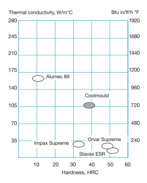
Note: Increasing alloying content gives a higher strength, but a lower thermal conductivity. However, this is only valid when comparing material within one material group i.e. steel must be compared with steel and copper with copper alloys.
