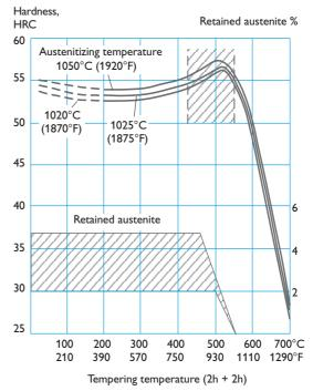
Above tempering curves are obtained after heat treatment of samples with a size of  $15 \times 15 \times 40$  mm, cooling in forced air. Lower hardness can be expected after heat treatment of tools and dies due to factors like actual tool size and heat treatment parameters.
