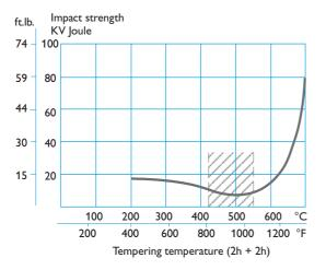
Tempering within the range  $425-550^{\circ}$ C (800-1020°F) is normally not recommended due to the reduction in toughness properties.
